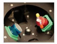
Push Open/Stop button on control panel. The "unlocked" indicator will illuminate. Turn latch counterclockwise to open lid. Place Restigen device into green bucket with side hubs oriented horizontally. Be sure the centrifuge is balanced with applicable counterbalance [60 mL Adjustable Counterbalance (Blue) or 60 mL Solid Counterbalance (Blue)] or a second full Restigen device. For the 30 mL device, use the purple 30 ml counterbalance
