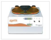
Close lid by rotating the lid latch clockwise. The "latched" indicator will illuminate. Set speed to 3200 n/min and time to 15 minutes. Press Start button. Once spin is complete, press Open/Stop button. Twist latch counterclockwise to open lid.
